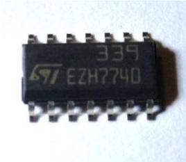
Quad analog comparator, U1, LM339A. Notice the faint writing on the chip. The “ST” logo at the left end should be positioned over the notch on the left side of the silk-screened outline of this chip. Position the chip over the outline, line up the leads with the pads, and solder one corner lead. Check positioning, reheat and adjust if necessary, then solder the remaining leads.
