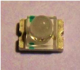
Examine the LED in the photo very carefully. You will notice a faint green band at the left of the plastic dome. That band **DOES NOT** mean it is a green LED! The green band on each LED marks the cathode (banded, or negative) end of the diode.
