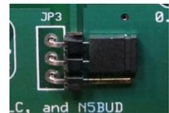
board, and the long pins will extend parallel to the board in the directions pictured. If you want to nip off a little bit of the long pins so that the jumper will fit flush, that's OK.
