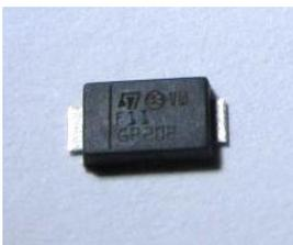
Rectifier diode, D1. Notice in the photo that there is a faint vertical line near the left edge of the part. That marks the cathode (banded) end of the diode. Be sure to install it on the board matching the orientation of the banded end of the silk-screened symbol.
