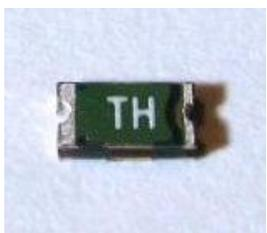
Resettable fuse, F1. Polarity is not a concern. It may be installed in either orientation.
