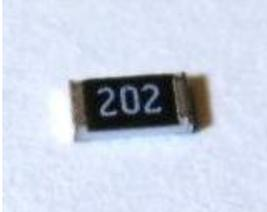
Six 2 K resistors. They look like the photo at left, and are to be installed on the top (silk-screened) side of the board along the left edge, just under the **BRARC** label.
